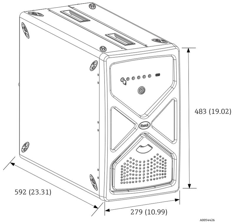
Figure 6. Raman Rxn2 analyzer. Dimensions: mm (in)
