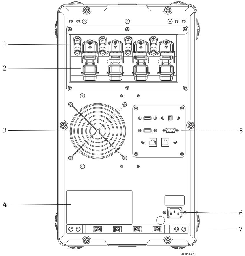
Figure 4. Rear panel of Raman Rxn2 four-channel analyzer
