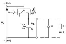
R<sub>L</sub> = Load resistance I<sub>L</sub> = Load current
